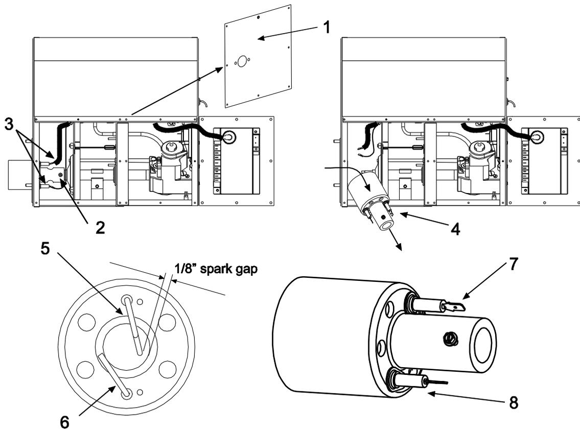
1. Disconnect electrical supply and Remove cover 1.
