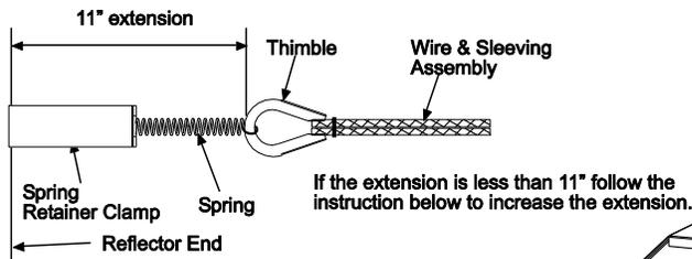
2. Tape one end of the sleeve to the burner box or use a marker.
