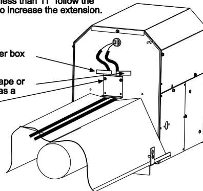
5. Pull one end of the sleeve and wire inside until the marker is raised by the total adjustment length. ie. if the extension is 10" then pull through 1" to increase the extension to 11".
