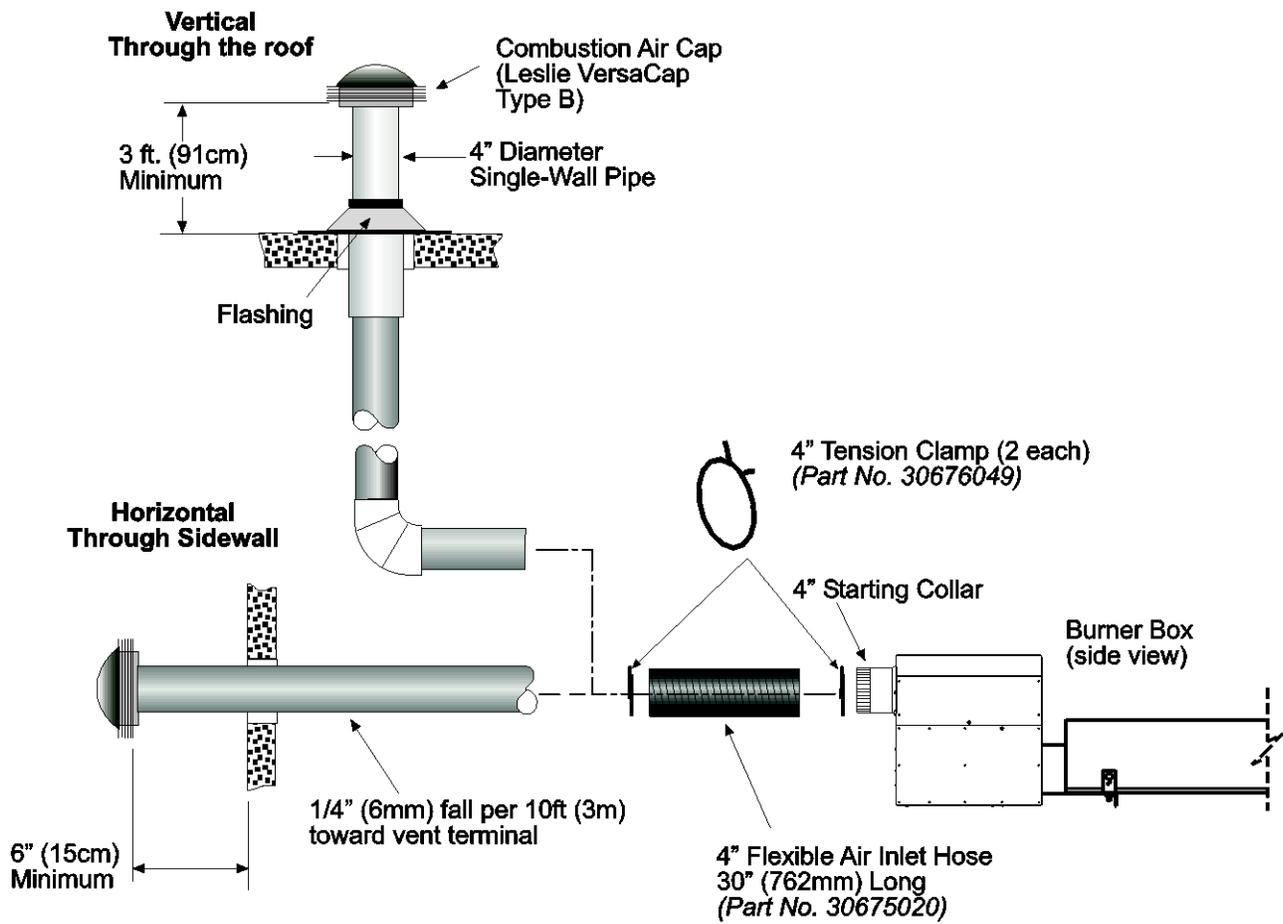
**! WARNING** All vent terminations and Combustion Air Intake Terminations must be at least 6" higher than anticipated snow depth.
