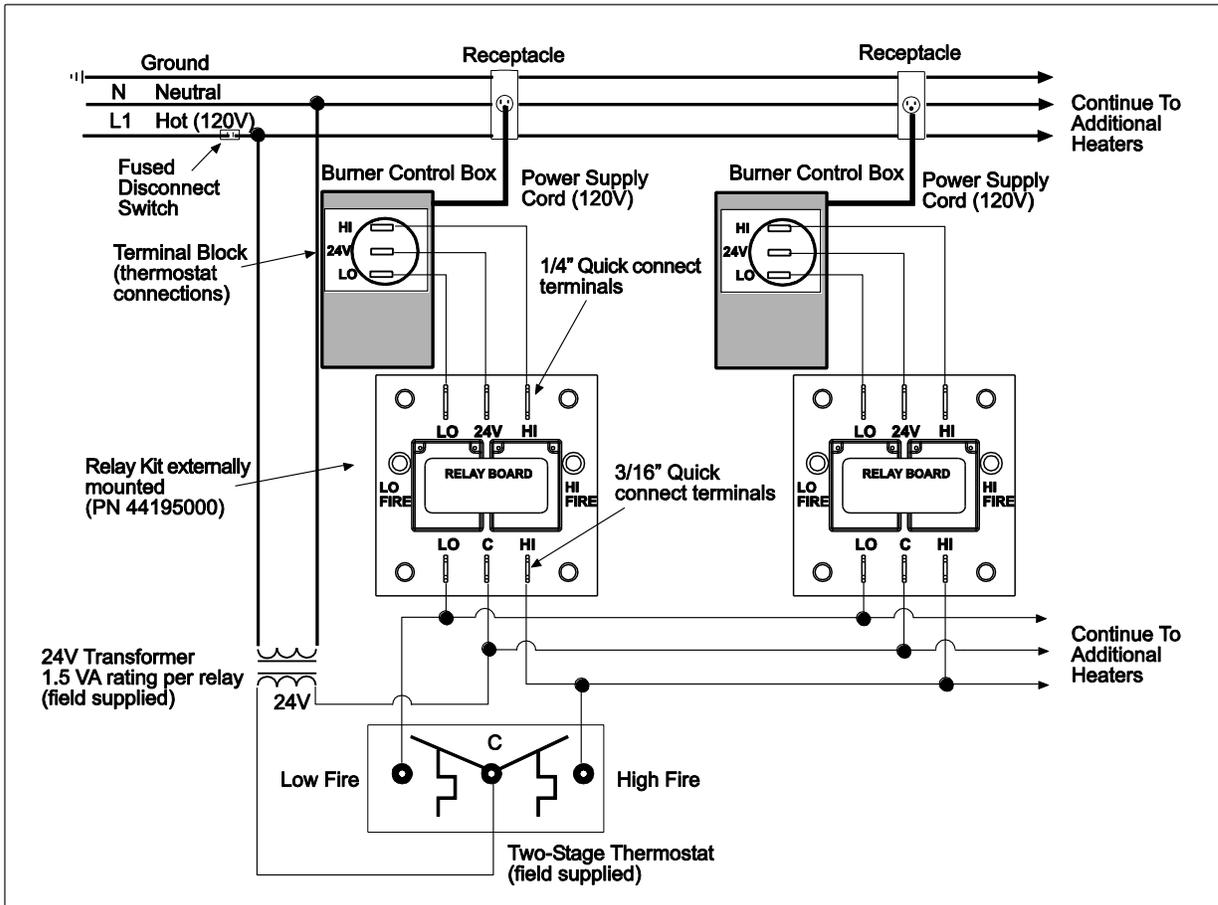
**C. LOW VOLTAGE (24V) 3 WAY MANUAL SWITCH CONNECTIONS – MULTIPLE HEATERS**
