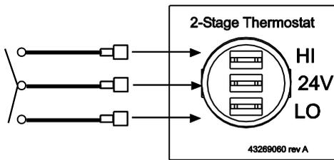
Use these three terminals for the 24V thermostat connection.
