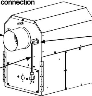
Liquid tight fitting must be tight to prevent ingress of moisture
