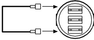
Jumper wire with 1/4" terminals pre-installed. Remove the jumper and use these two terminals for the 24V thermostat connection if required.
