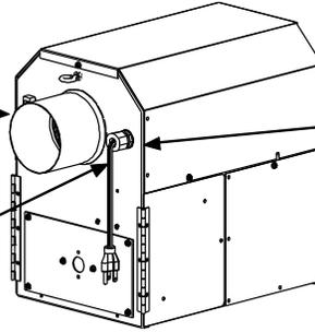
Liquid tight fitting must be tight to prevent ingress of moisture in harsh environments.
