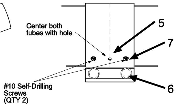
4. Slide the next tube into the coupling.
